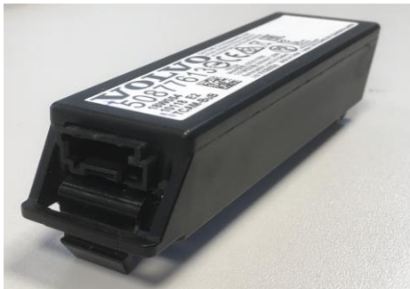
Figure: Backup Battery
